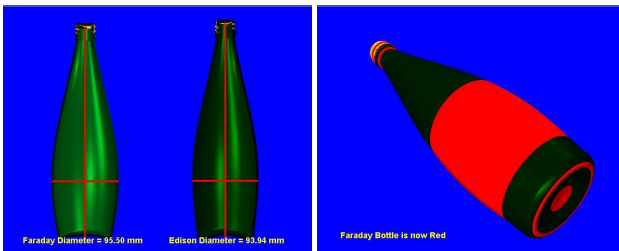
Figure 2: Comparing Dimensions (part of Faraday's case) and Shape (for Edison's case) using the Virtual Bottles.
