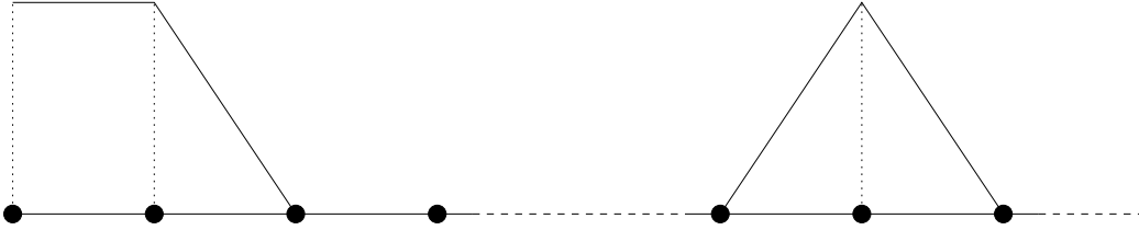
Figure 1: Test functions for the recovery of U via mass conservation in one dimension which are compatible with strong imposition of Dirichlet boundary conditions.
