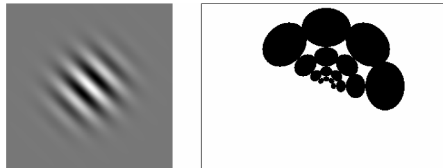
Figure 8. (a) Gabor filter in spatial domain (real part), (b) Filter bank in spatial-frequency domain (half peak)
