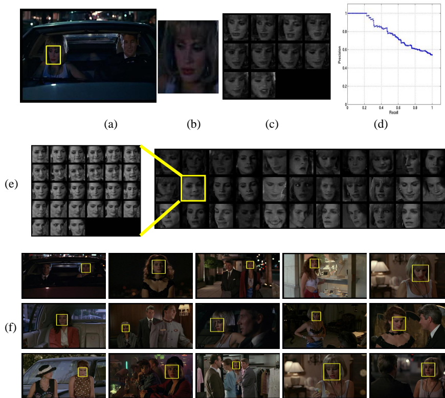
Fig. 7. Example retrieval of the main character from the movie ‘Pretty woman’. (a) The query frame with the query face outlined in yellow. (b) close-up of the face. (c) The associated set of 10 face detections in this shot. (d) Precision-Recall curve. (e) Right: the first 33 retrieved face sets shown by the first face detection in each set. Left: example of a retrieved face set. (f) Example face detections from the first 15 retrieved face sets superimposed on the original frames. Note the extent of pose, lighting and expression variation among the retrieved faces. For this character, the number of relevant face-tracks in the ground truth set is 145.
