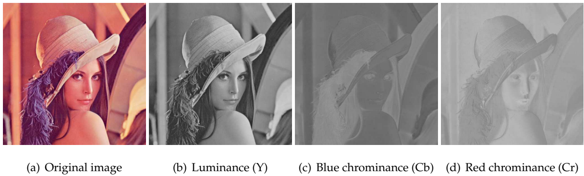
Figure 3.1: The above figures show how an image is represented in the YCbCr colour space. The original image is shown on the left along with each of its three channels, a luminance channel and two chrominance channels containing blue and red levels.
