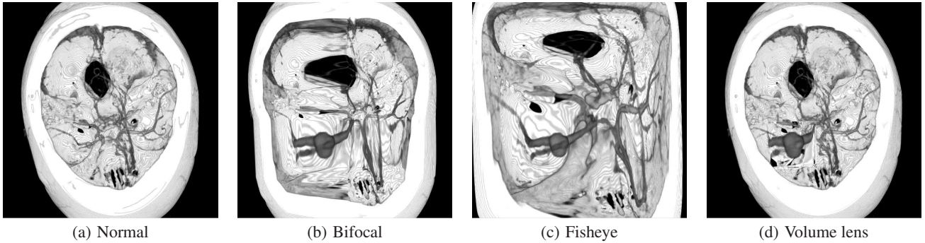
Figure 1: Mapping effects in 3D: (a) no effects; in (b) the bifocal effect helped to distinguish between the focus and context regions; in (c) the fisheye effect better preserved the spatial relationships of the data; in (d) the volume lens effect produced a magnified view of just the focus region.
