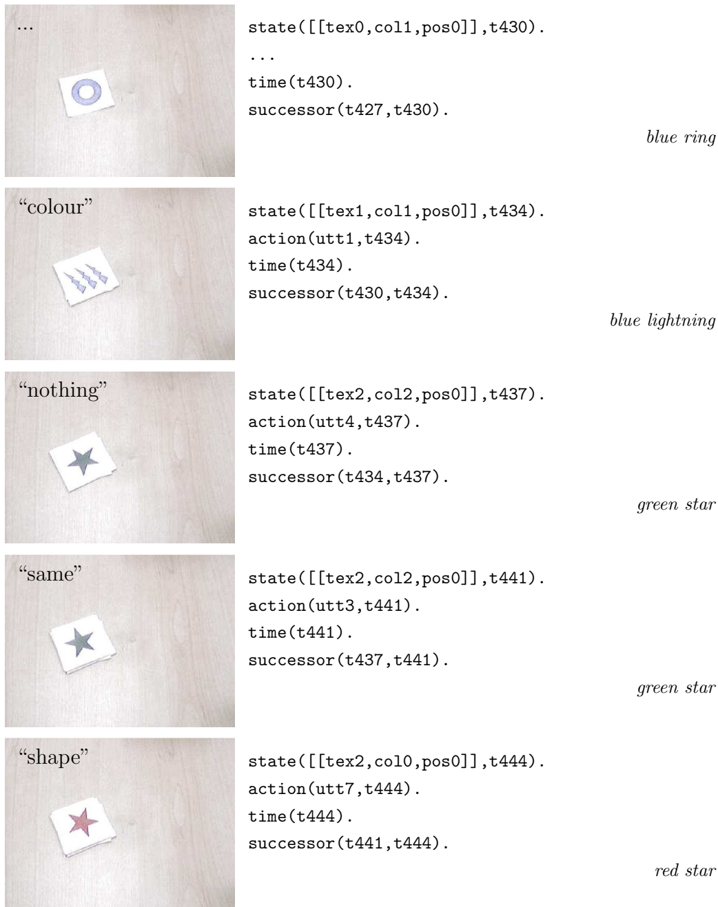
Fig. 16. Example audio-visual inputs and corresponding symbolic data representation for the game SNAP2.
