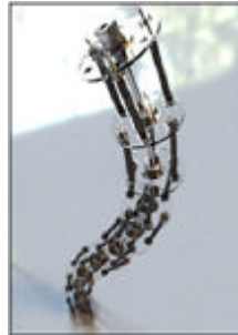
Figure 1. Snake robot. Copyright: Chris Forbes, NTU
