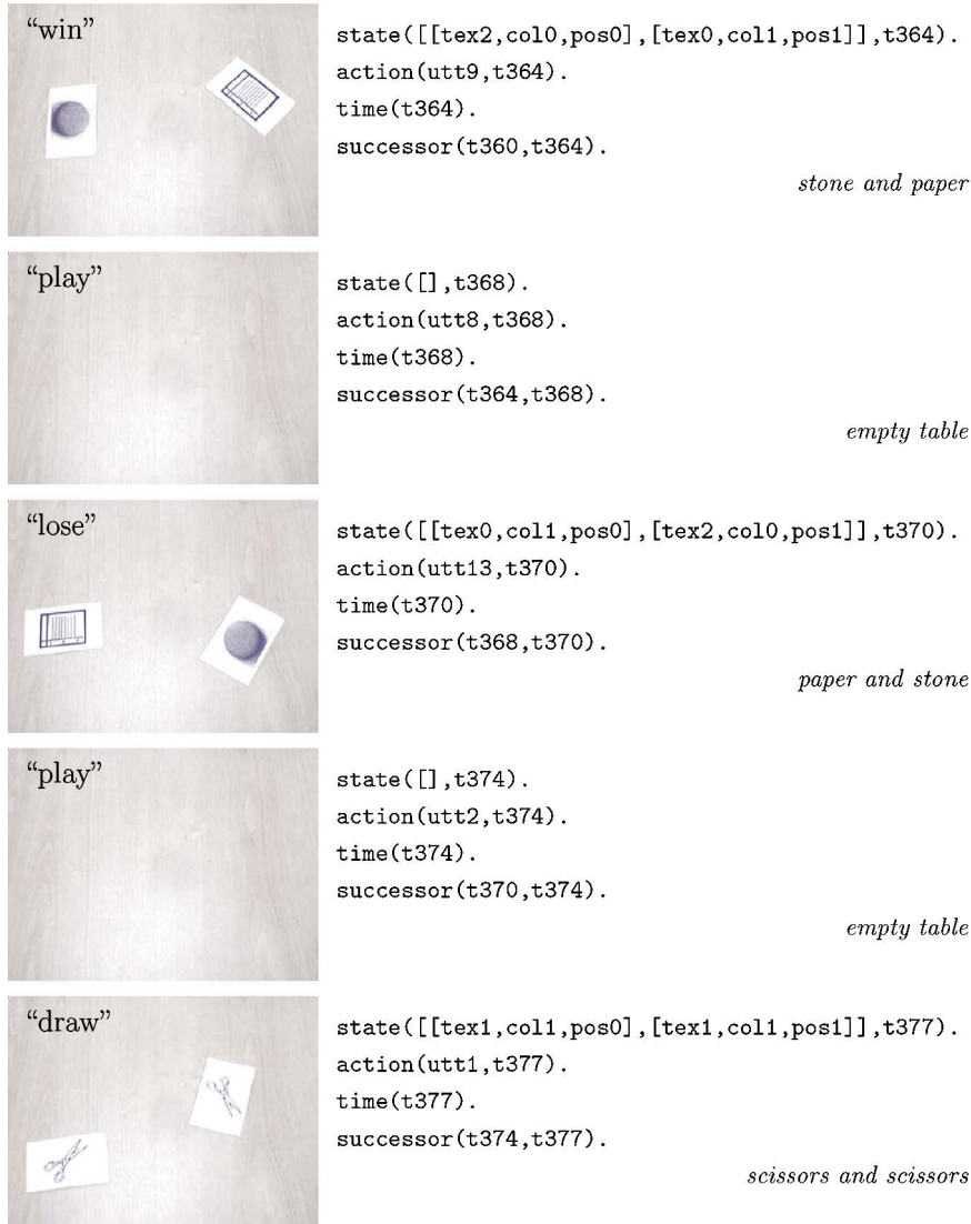
Fig. 18. Example audio-visual inputs and corresponding symbolic data representation for the game PSS.
