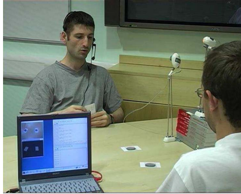
Fig. 1. Example of the data collection phase. A game is played on the table between two players. One camera points down at the table, and another captures the face of the participant to be replaced by the synthetic agent. The audio is captured by a microphone worn by this participant.
