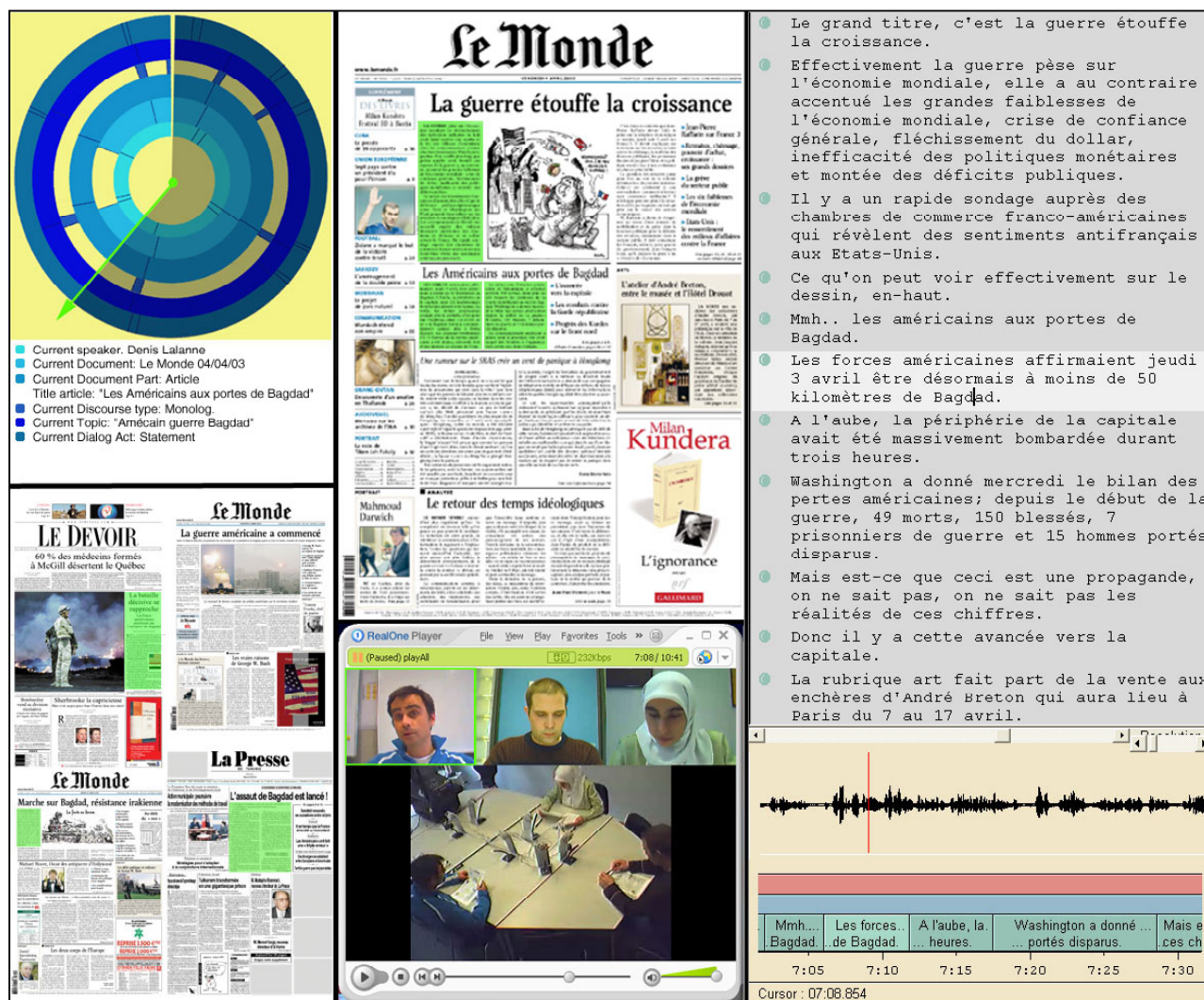
Figure 4: A mock-up of the minutes application as we envision it, with the following components: the kaleidoscope visualization, the document in focus, the audio/video movies, the structured speech transcription and the audio signal. All those representations are synchronized.
